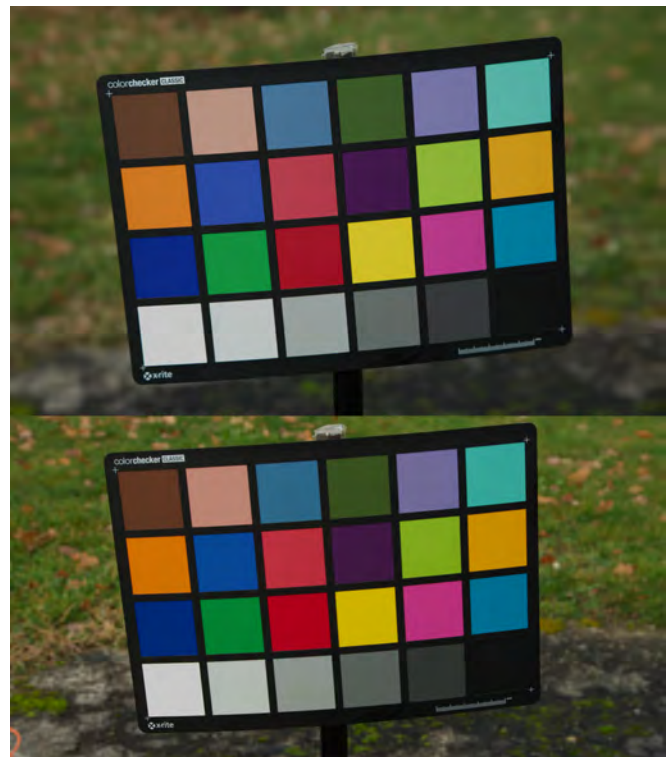
Figure 16. Recordings of a ColorChecker under the same lighting conditions. Top: rawtoaces , bottom: REDWideGamutRGB
