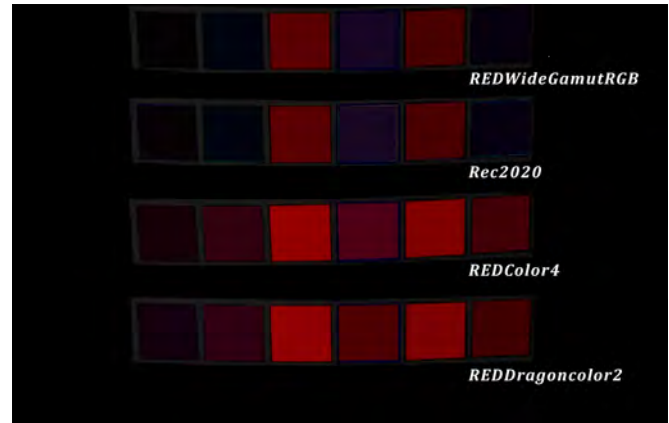
Figure 14. Differences between ACES RGB data set of selected ColorChecker patches and ACES IDT converted RED Scarlet-X recordings
