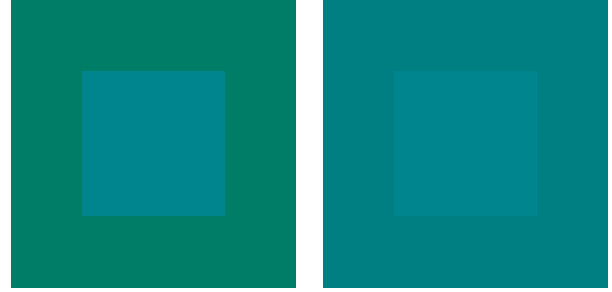
Figure 3. Two spectral samples that are device parameric under tungsten light are shown. The inner rectangle shows the reproduced color of the camera after a linear color correction. The outer rectangle shows the color as seen by the CIE 1931 2° standard observer.
